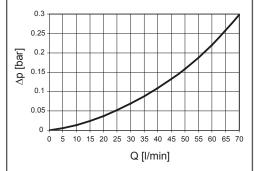
The gradient coefficients in mbar/ (I/min) apply to mineral oils with a kinematic viscosity of 30 mm<sup>2</sup>/s. The pressure drop changes proportionally to the change in viscosity.
